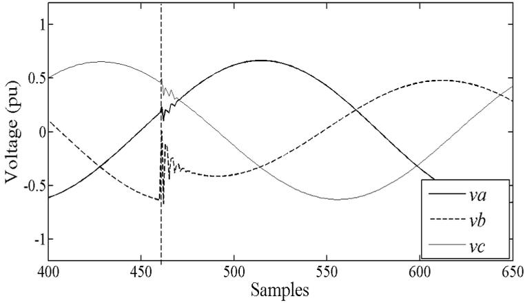
Fig. 9. Three phase voltage of single phase fault
