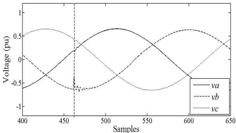
Fig. 11. Three phase voltage of single phase HIF
