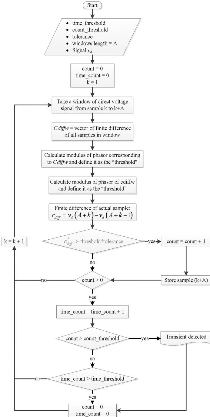
Fig. 3. Full algorithm for the transient detection
