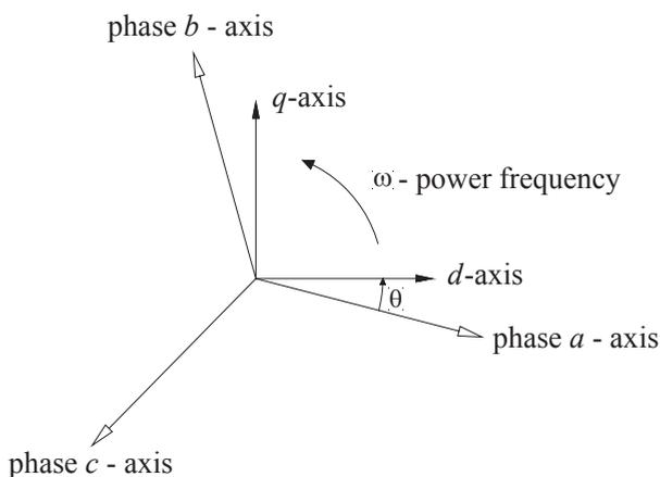
Fig. 1. Diagram of a three-phase system and  $dq$  components
